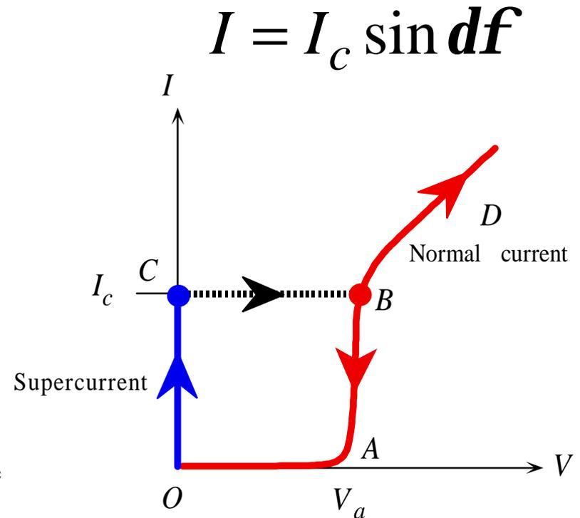
Fig. 8 58: (a) A Josephson junction is a junction between two Fig. 8 59:  $I$ - $V$  characteristics of a Josephson junction for positive
